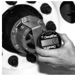
Install DataTrac® PRO on wheel end.
